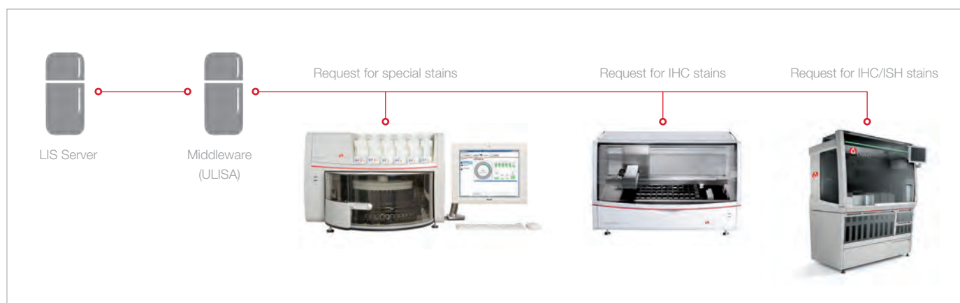
Figure 10.5 Integration from a Laboratory Information System (LIS) to the stainer instruments can be accomplished through a single point of connection using an integration module, e.g. the Universal LIS Agent (ULISA). The ULISA manages communication with a LIS server and provides the various instruments with the data received.
