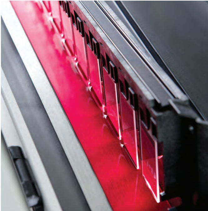
Figure 3.2 Dako PT Link is a water bath method for antigen retrieval
